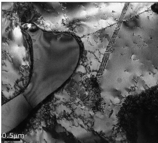
Fig. 4. TEM bright-field image of AISI 347 heat affected zone.
